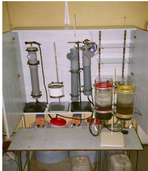
Figure 5.4. Anaerobic-aerobic textile wastewater treatment's laboratory system.
