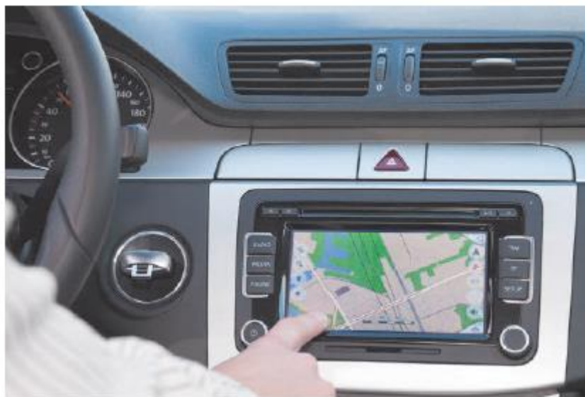
Figure 1-11. Portable and built-in navigation devices have embedded operating systems (Source: Brainpulse, Creative Commons License).
